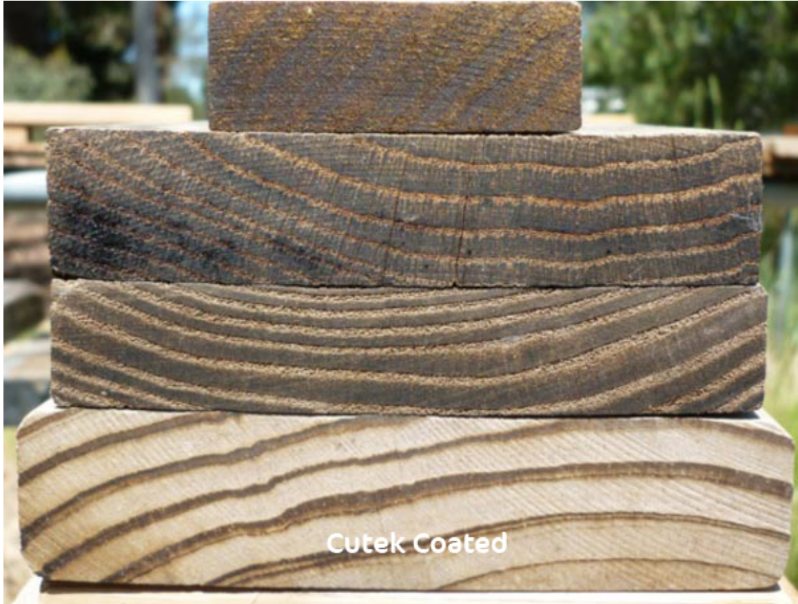
Picture 3 Several species of lumber which were dip coated once in CUTEK™EXTREME (one end of the board only). The other end was left uncoated. This picture of the dipped ends was taken 12 months after coating.
