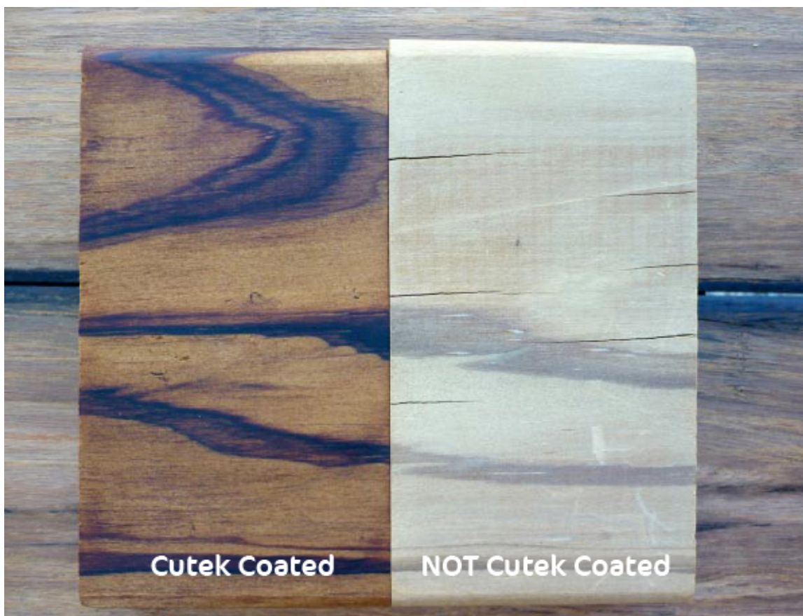
Picture 1. Thermally treated Southern Yellow Pine six weeks after the piece was cut in half, and one side (left) was dipped once in clear CUTEK™EXTREME . The picture shows swelling and fading in the uncoated portion. These pieces were both left in full sun and rain exposure
